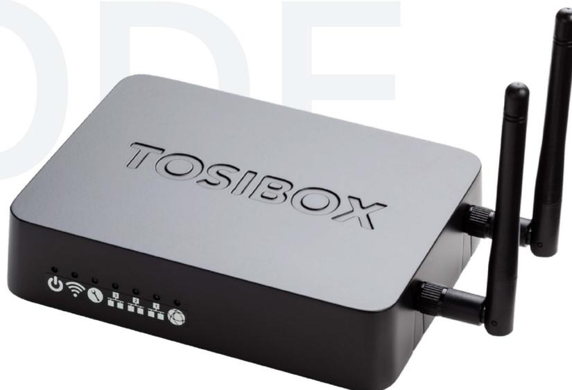
TOSIBOX® Lock 150 is an industrial router with firewall and secure Plug & Go™ connectivity. It serves as an endpoint for secure remote connections.
